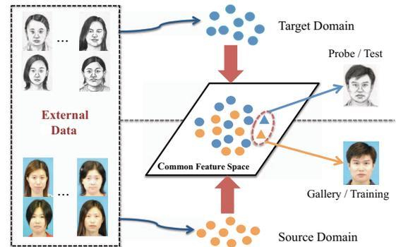
Fig. 1. Illustration of domain adaptation for heterogeneous face recognition. Note that the external face images applied for associating source and target domains are collected from subjects *not* of interest (in circles), while the gallery and probe images are from the subjects to be recognized (in triangles).
